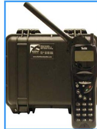
Larger offices may want to consider a fixed satellite phone unit, which can provide satellite-based telephone using an outside antenna and any analog phone. While somewhat more expensive than a handheld satellite phone, this system also requires a backup power supply and may therefore be of limited utility in worst-case scenarios.
